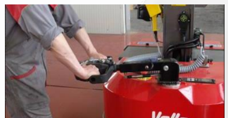
180° steering helm powered by electric motor with 180° rotation for maximum manoeuvrability
