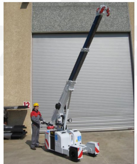
Fully hydraulic telescopic boom
