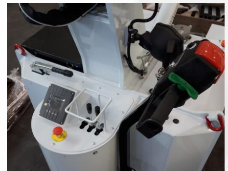
180° steering helm powered by electric motor with 180° rotation for maximum manoeuvrability
