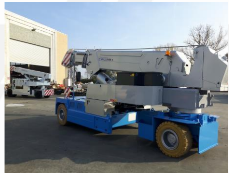
Extendable chassis to increase lifting capacity
