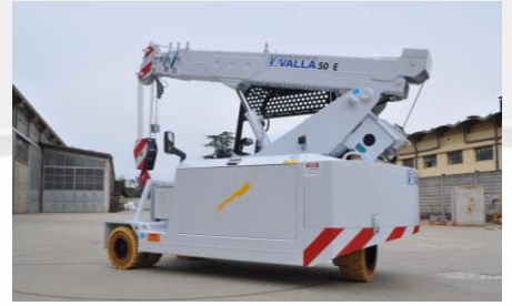
Rear steering with 180° rotation for maximum manoeuvrability
